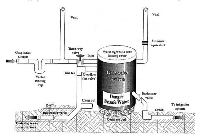
Figure 1-Graywater System Single Tank-Gravity (conceptual)
