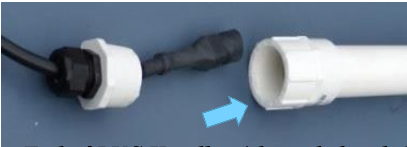
Top End of PVC Handle with newly bonded adapter
