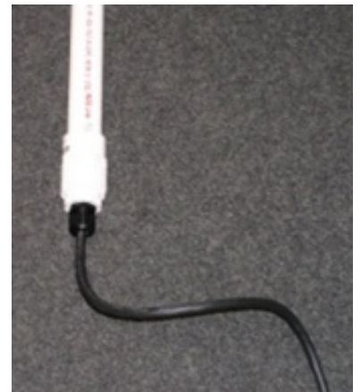
PHOTO 25 WATERTIGHT FITTING INSTALLED ON HANDLE
